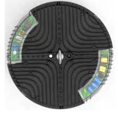
Compared with the original driver installation on the heat sink, the driver install on the side of the heat sink is much better.
